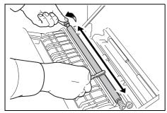
Run the brush from side to side along the transfer roller as shown, rotating by the gear at the end, to remove any soiling.
